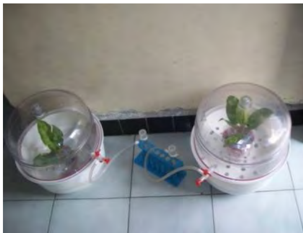
Plate 3: Exposure of Aglaonema commutatum in the exposure chamber
