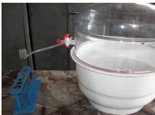
Plate 2: Exposure chamber, vacuum desiccators
