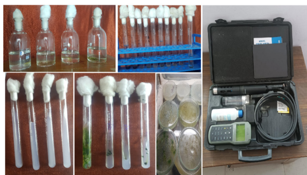
Fig. 3: Collected samples and experimental setup with water analyzer (HANNA HI98196).
